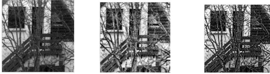
Fig. 22 SWIR images; non processed on left, CLAHE in the middle, BILATERAL on right
